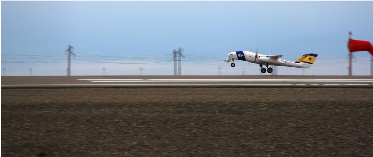
The University of Alaska SeaHunter UAS takes off from Ugnu-Kuparuk Airport in Alaska, equipped with the NOAA *miniFlux* sensor (under the nose) to make measurements of atmospheric state and turbulence over the Beaufort Sea during the SODA field campaign.
