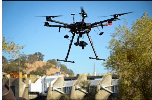
**Matrice 600 UAS platform integrated with Nano hyperspectral (270 band) sensor.**
