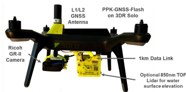
**Three 3DR Solo UAS will be autonomously flown in formation flight. Each Solo is configured with Ricoh GR-II camera, 850nm Lidar, and PPK.**
