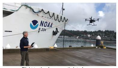
Flight testing for magnetic interference.
