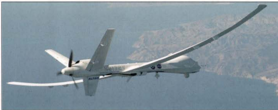
Fig. 1. The Altair in flight at three-kilometer altitude over the Channel Islands National Marine Sanctuary off the coast of California on 16 November 2005. The electro-optical infrared sensor protrudes below the forward fuselage.
