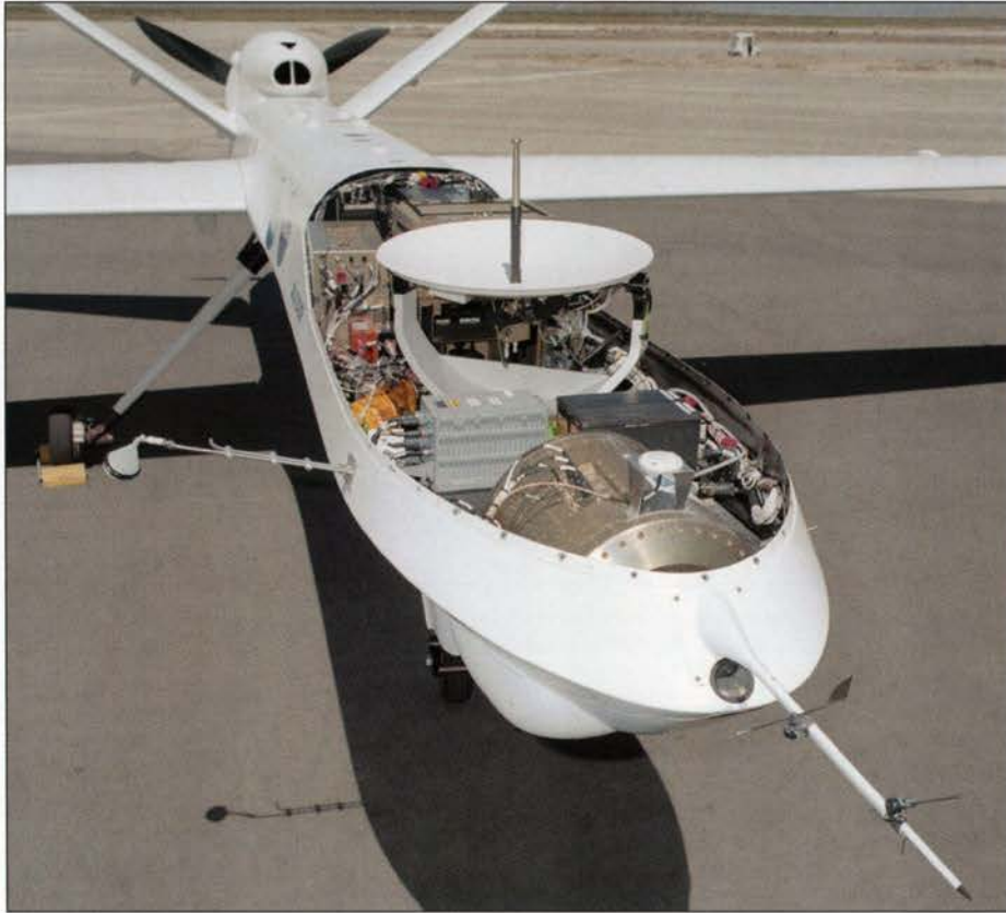
Fig. 2. The Altair with its fuselage payload bay open at Gray Butte Airfield in April 2005. The sampling instruments are located inside the fuselage nose along with the gimbaled satellite antenna. The gas-sampling probe is visible on the left of the fuselage in this view. The small forward boom is used for sensing wind direction. The small opening at the tip of the nose is a camera port used by the pilots. Also visible above the rear fuselage is the engine intake and propeller.
