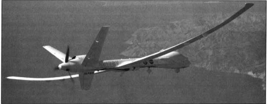
Fig. 1. The Altair in flight at three-kilometer altitude over the Channel Islands National Marine Sanctuary off the coast of California on 16 November 2005. The electro-optical infrared sensor protrudes below the forward fuselage. Original color image appears at the back of this volume.
