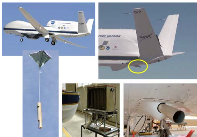
Figure 1. (Clockwise from top left) Global Hawk; close-up of Global Hawk with dropsonde eject tube, circled in yellow (photo courtesy of NASA); close-up of dropsonde launch tube (photo courtesy of NASA); dropsonde dispenser and launch assembly; dropsonde with parachute.
