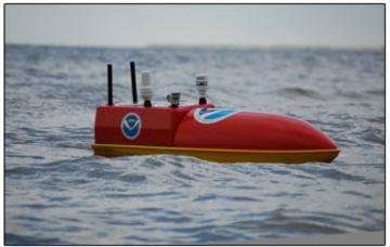
EMILY, a 65-inch water-tight craft, is one of the newest of NOAA's hurricane research platforms. Outfitted with a satellite link, camera, battery and gasoline motor, and a variety of snesors, EMILY will collect sea-level data from within a hurricane beginning with the 2012 hurricane season. Credit: Hydronalix, Inc.
