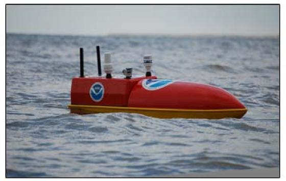
EMILY, a 65-inch watertight craft, is one of the newest of NOAA's hurricane research platforms. Outfitted with a satellite link, camera, battery and gasoline motor, and a variety of sensors, EMILY will collect sea-level date from within a hurricane beginning with the 2012 hurricane season. Credit: Hydronalix Inc.
