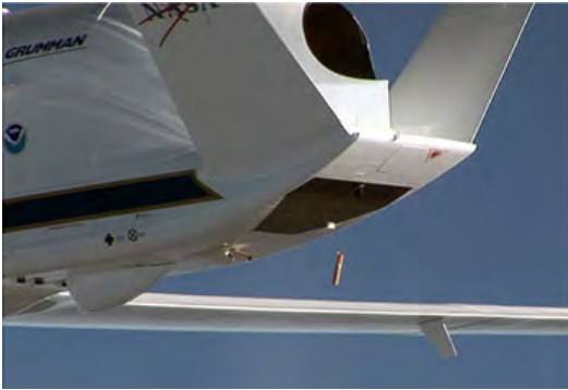
A dropsonde is released from one of NASA's Global Hawk aircraft. The paper-towel-sized instrument contains sensors that measure precise location (and therefore wind), temperature, humidity, and pressure. Credit: NASA
