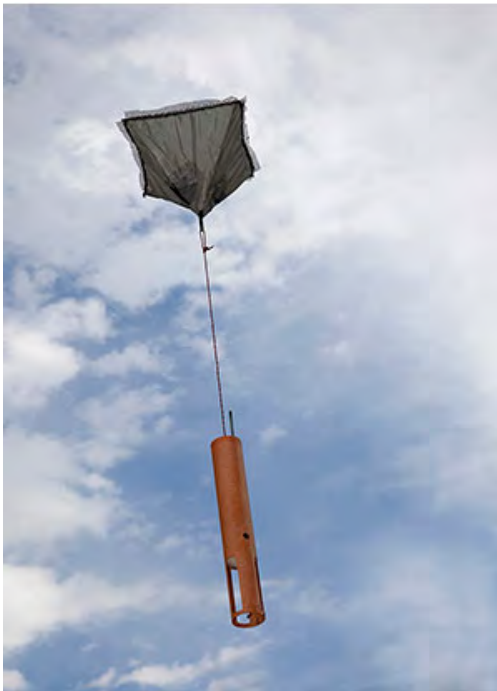
A dropsonde is released from one of NASA's Global Hawk aircraft. The paper-towel-sized instrument contains sensors that measure precise location (and therefore wind), temperature, humidity, and pressure. Credit: NASA
