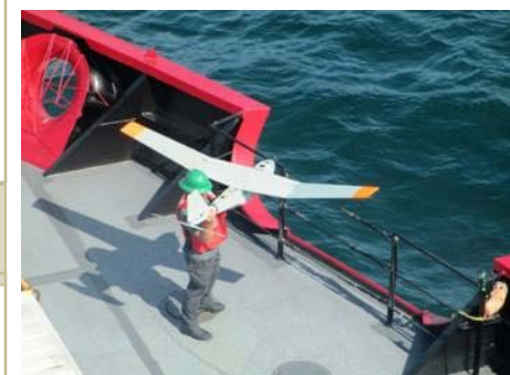
Puma launches from the USCGC Icebreaker Healy north of Oliktok Point, AK, during 2015 Joint Search & Rescue Exercise conducted with other manned and unmanned aircraft. Source: USCG
