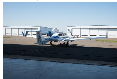
The Aurora Flight Sciences Centaur Optionally Piloted Aircraft was successfully tested for gravity sampling missions with SBIR funding. Source: Aurora Flight Sciences
