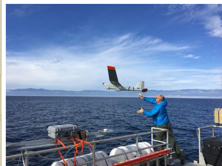
Puma launches from the NOAA R/V Shearwater at the Channel Island National Marine Sanctuary for testing of the autonomous net-capture system in preparation Arctic Shield 2018. Source: NOAA
