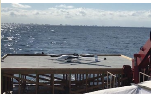
The L3Harris FVR-55 fixed wing hybrid quadrotor during launch and recovery exercises off NOAA Ships
