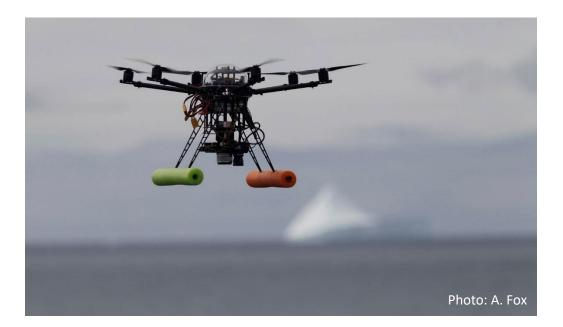
The APH-28 unmanned aerial system (Aerial Imaging Solutions, LLC) surveying Antarctic fur seals near Cape Shirreff, Livingston Island. Payload: downward facing micro 4/3 format digital camera with a laser altimeter.
