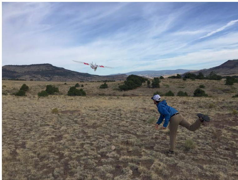
Fig. 1. A University of Colorado Boulder UAS is launched to measure atmospheric thermodynamic state and winds during LAPSE-RATE.
