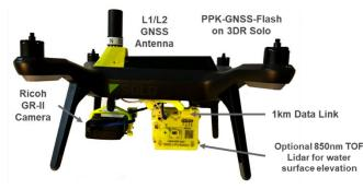
Three 3DR Solo UAS will be autonomously flown in formation flight. Each Solo is configured with Ricoh GR-II camera, 850nm Lidar, and PPK.
