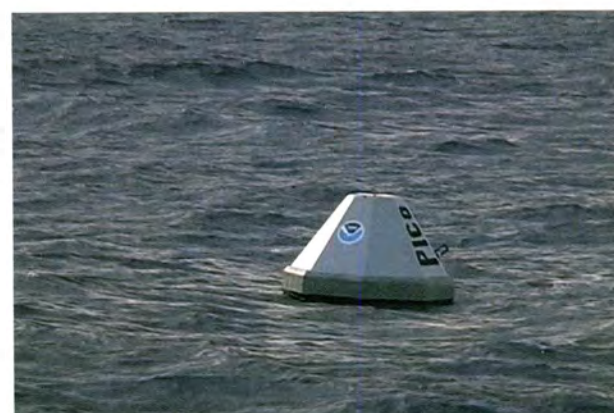
FIG. 7. Two views of the PICO buoy: (a) being readied for deployment, and (b) as deployed. It is designed to be easy to deploy, inexpensive, and require significantly less on-site routine maintenance than the TAO buoys.
