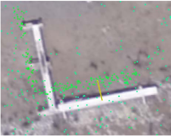
Figure 35. Boardwalk in area of interest 2. Returns from the wet mud around the planks made returns (green dots) scarce and the boardwalk more apparent in the lidar.
