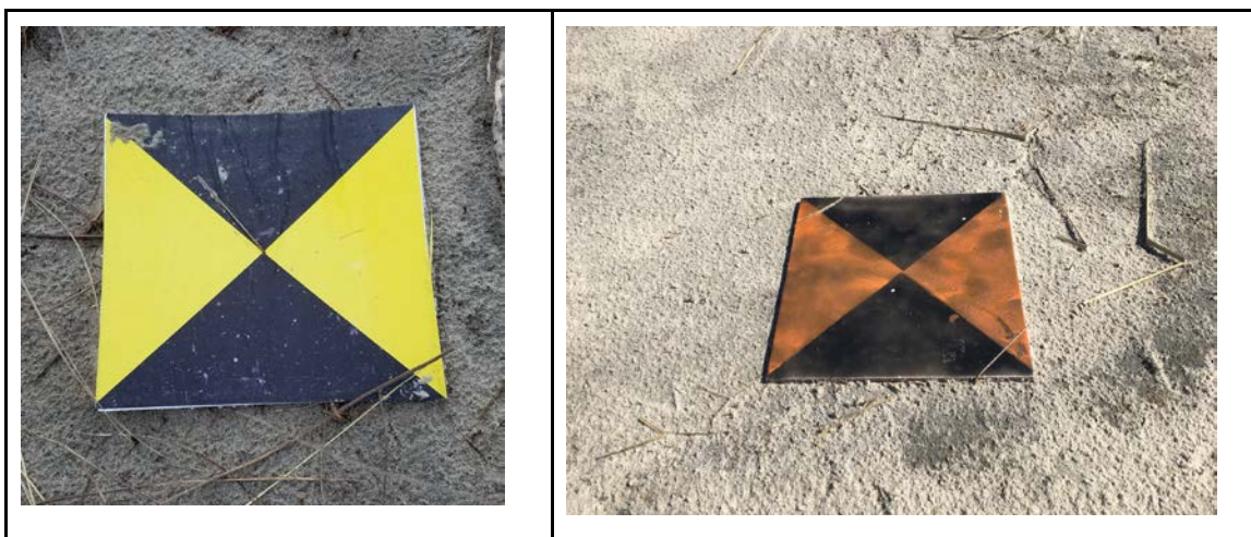
Figure 7. Examples of targets used. On the left is a foam-backed target and on the right is a floor-tile target. All targets had the potential for coverage by sand, which may have made their identification harder.
