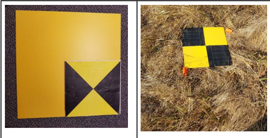
Figure 45. The image on the left shows the size of the targets used at Jacques Cousteau compared to the new targets before Duck tape patterning. The image on the right shows the final targets as deployed in the uplands at Rush Ranch.
