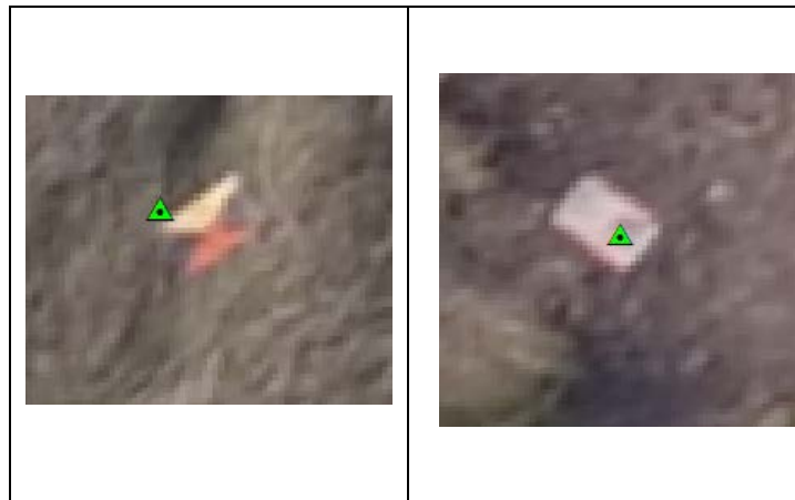
Figure 19. Examples of photo-id targets in the UAS imagery with the surveyed location of the target shown as a green triangle. If the imagery georeferencing were perfect, the green triangle would be in the center of the target.
