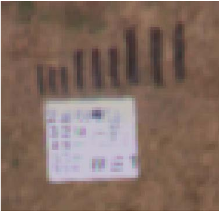
Figure 51. USAF-1951 chart as seen in the mosaicked imagery. No stretch was applied.
