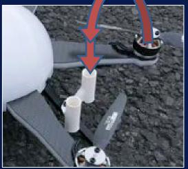
Sensors are sheltered and mounted in the rotor downwash
