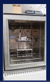
Control Calibration Chamber: iMet sensors sampled every second taken from -60C to +40C over a period of 10h meet NOAA's accuracy and response time specs
