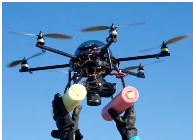
APH-22 hexacopter with gimbal camera for photogrammetry being hand-launched (J. Durban, H. Fearnbach, SWFSC)
