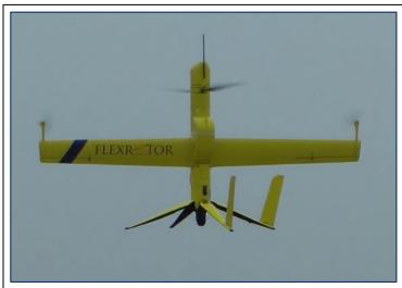
Actaea lifts off into gray and rainy skies at the start of its 32-hr flight. Legs are about to fold for transition to wing-borne flight.
