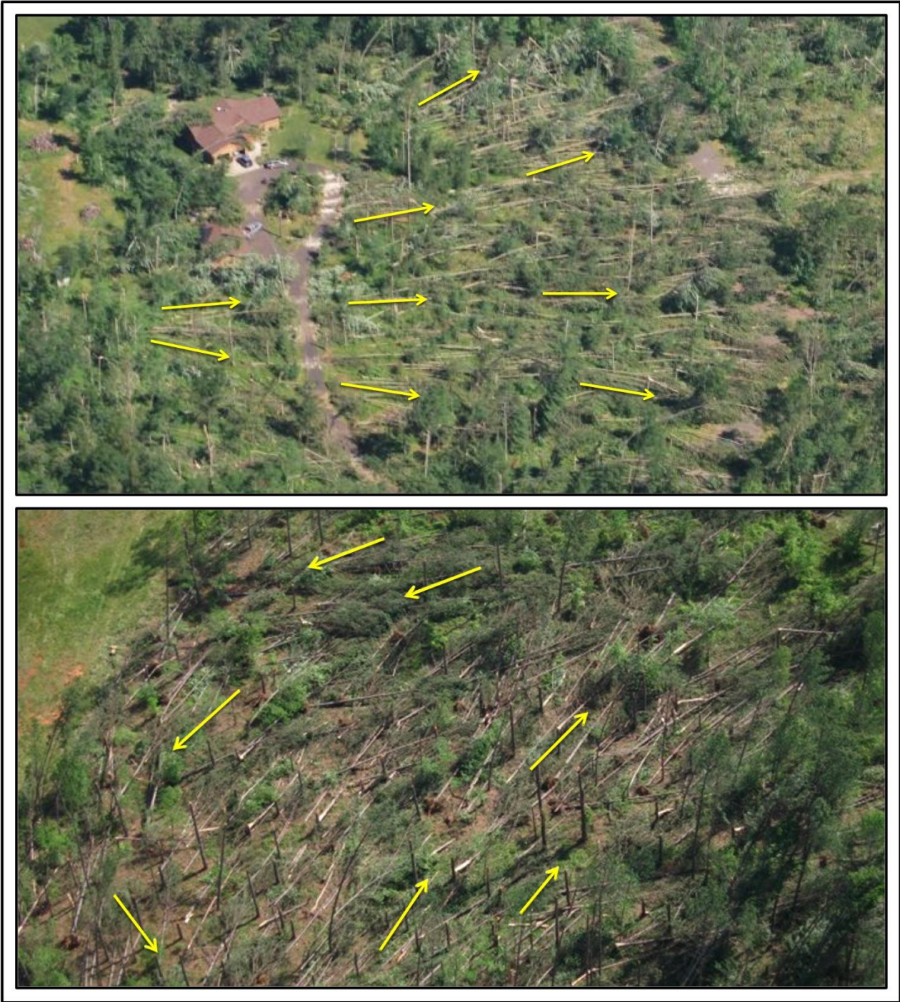
Figure 4. Straight-line wind damage is often characterized by a fanned out tree-fall pattern (top), whereas, a convergent or “cross-over” tree-fall pattern is often indicative of a tornadic circulation (bottom). Images provided, courtesy of NWS WFOs in Duluth, MN, and Huntsville, AL, respectively.
