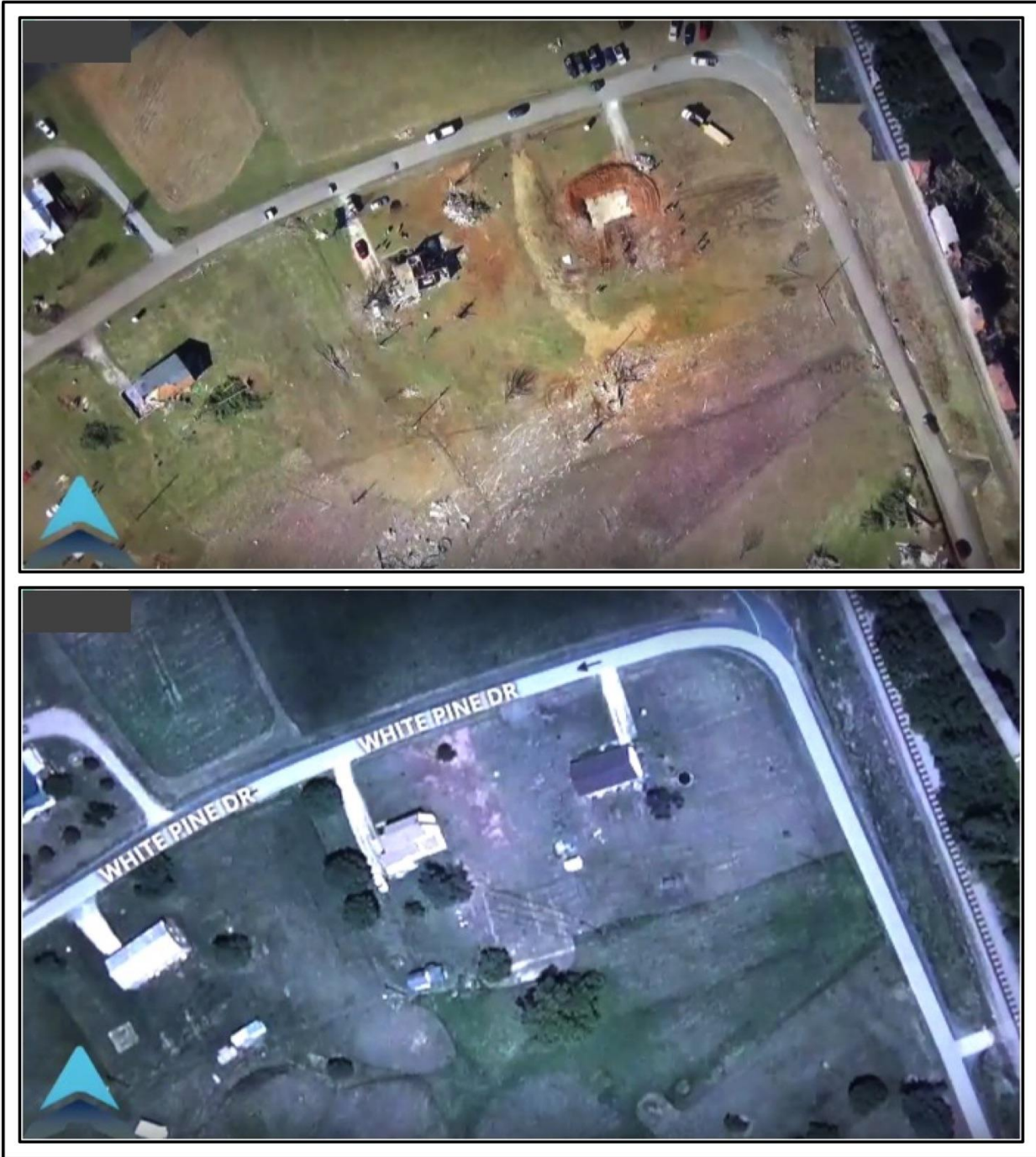
Figure 19. The orthomosaic image captured in Appomattox County, VA, (top) is compared to the same scene provided in Google Earth (bottom) by toggling back and forth between the base map and the orthomosaic. Imagery produced by Autonomous Flight Technologies, Inc. and provided courtesy of NWS Blacksburg.
