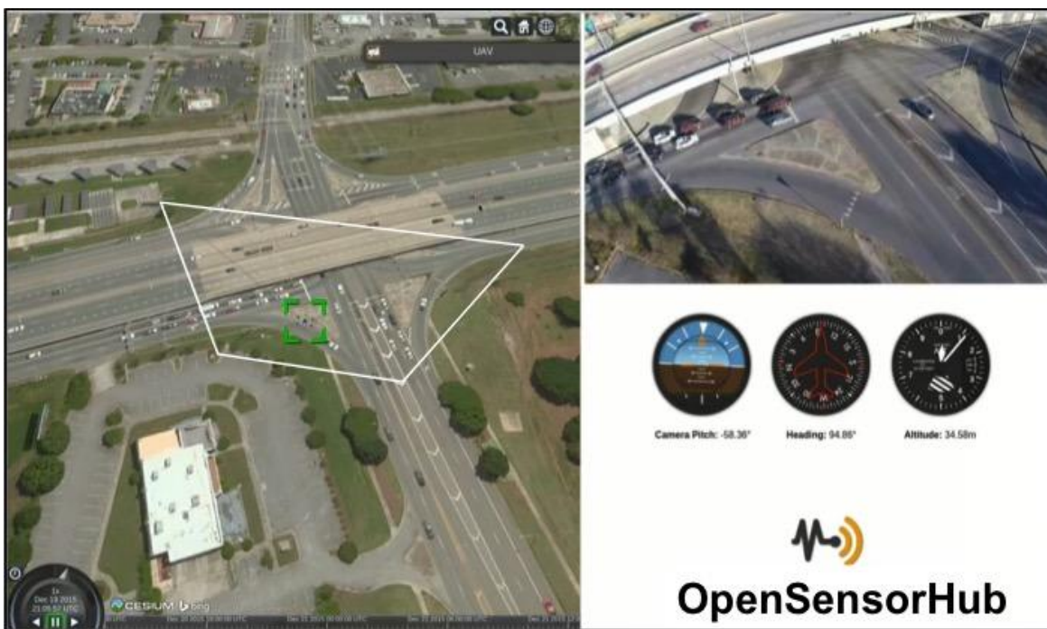
Figure 24. Sample screenshot of OSH application in which FMV imagery is displayed in real time at the top-right, while the UAS and camera payload positional information is provided on a static base map to the left.
