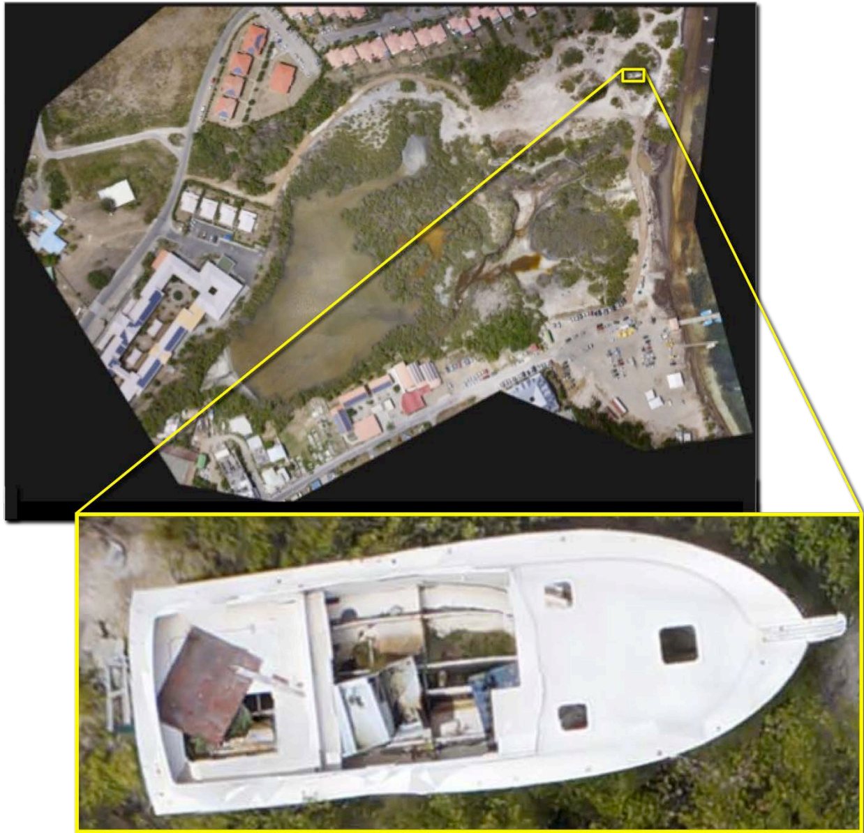
Figure 18. A high-resolution orthomosaic image, such as this, can provide a broad overview of an area, complete with geographic coordinate information, and when zoomed in, it can facilitate discovery of detailed features within the imagery. Dataset provided courtesy of Skylab Production.
